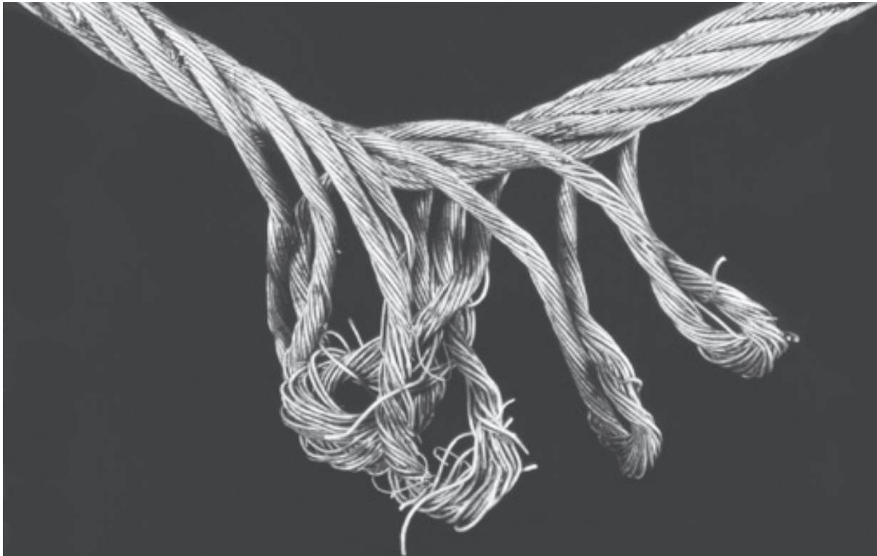
Fig. 37: Surplus length of the outer strands caused by unlaying the rope
