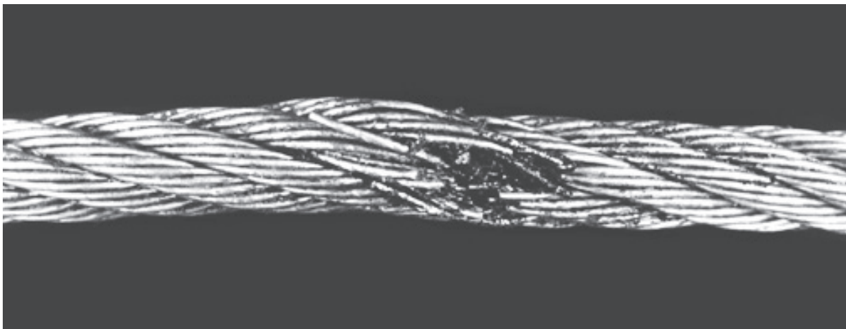
Fig. 4: A local concentration of wire breaks
