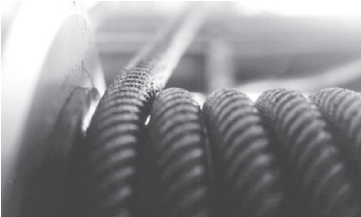
Fig. 44: Under the influence of a fleet angle, the wire rope is pulled against a neighbouring wrap. The outer wires will be damaged at the point of contact.
