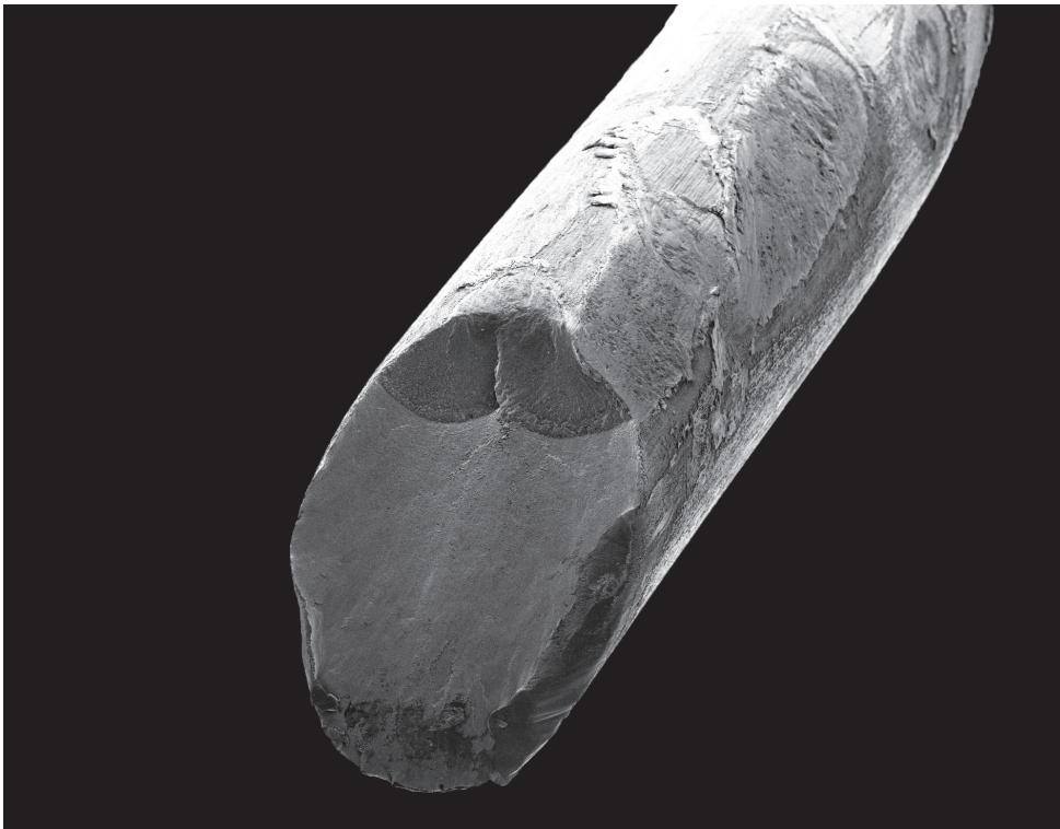
Fig. 18: An internal round wire. Two adjacent fatigue cracks have started at points of contact with neighbouring wires. The wire finally failed in shear. (approximate magnification \times 15 ).
