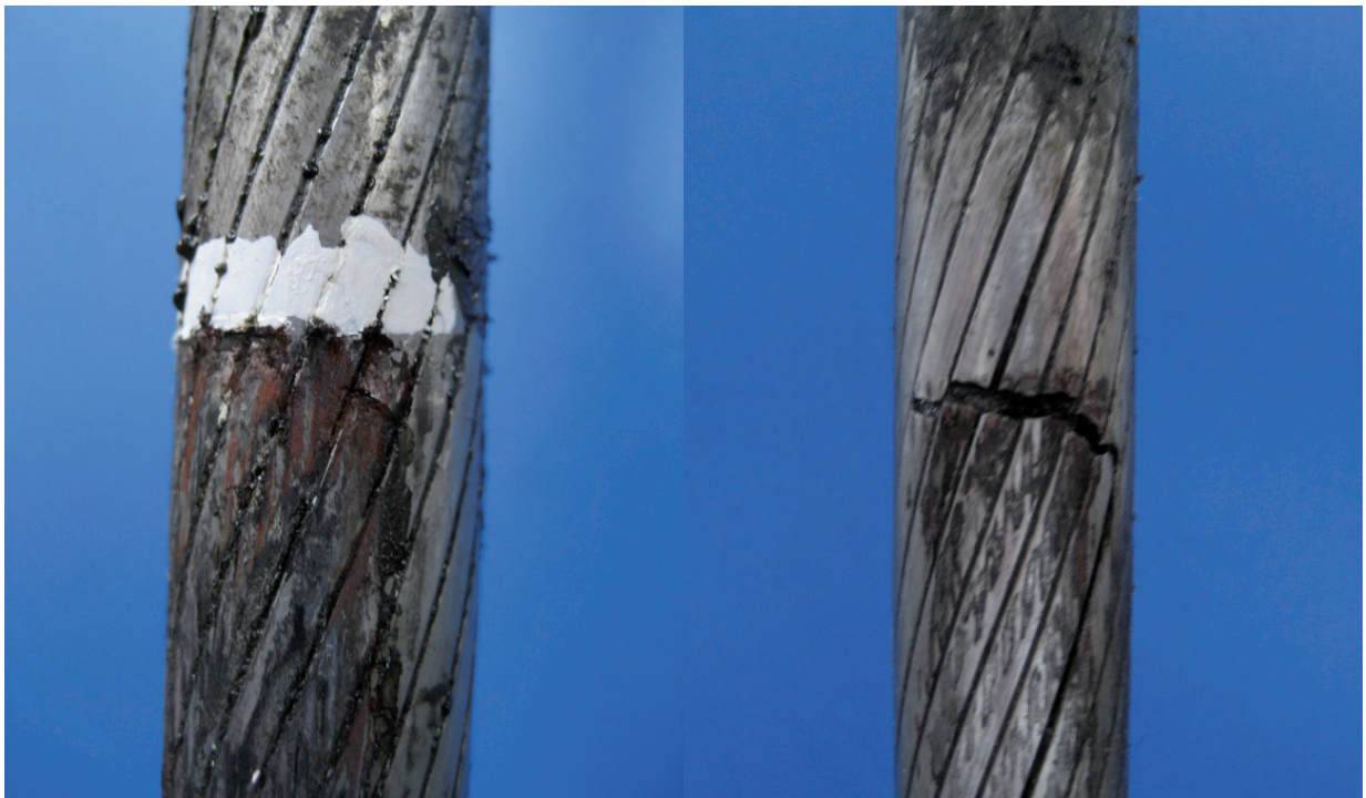
Fig. 14: Clamp upper exit point (‘front’ (left) and ‘back’ (right)). Note the wire breaks and fretting rouge at the position of the rope just inside the clamp (the edge of the clamp is marked on the front view with the white paint). It is thought that the marks on the Z wires (back view) are from the damage to the clamp from the previous tests on the six-strand rope.
