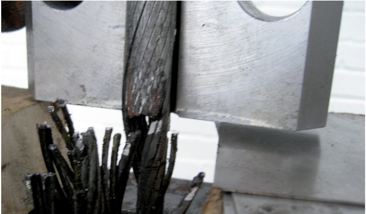
Fig. 13: Clamp lower exit point at which the main failure occurred. Note the Z wires which were at the ‘sides’ of the clamp groove have not failed. Note also the fretting rouge at the position of the rope just inside the clamp.
